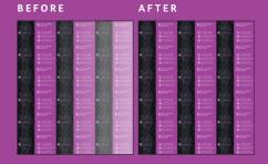
**Auto Density Uniformity Adjustment:** Lead-to-trail edge and inboard-to-outboard density uniformity.
